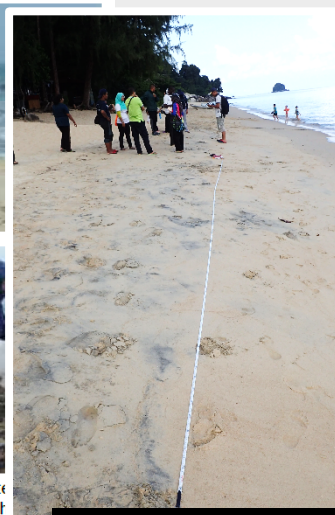
Figure 4.11 NOAA protocol for shoreline monitoring. Shoreline section (100 m) displaying perpendicular transects from water low tide to the first barrier at the back of the shoreline section. Red circles indicate marked GPS coordinates. Shoreline width location and number of GPS coordinates. Figure not to scale. (from Lippiatt et al. 2013, images ©NOAA).
