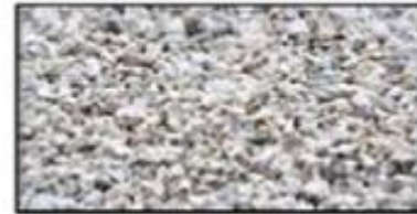
Stone aggregate heated to around 160-170°C
